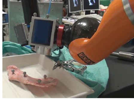
Robot Assisted Laser Bone Cutting Wörn, Raczkowsky, KIT EU Project AccuRobAs: Accurate Robot Assistant
