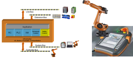
KRC Nexxt Controller Architecture / Safety Regulation
