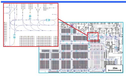
Segmented Roadmap. A path is given as a set of segments to be tracked
